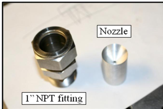
Fig. 18. Exit NPT fitting and nozzle.
