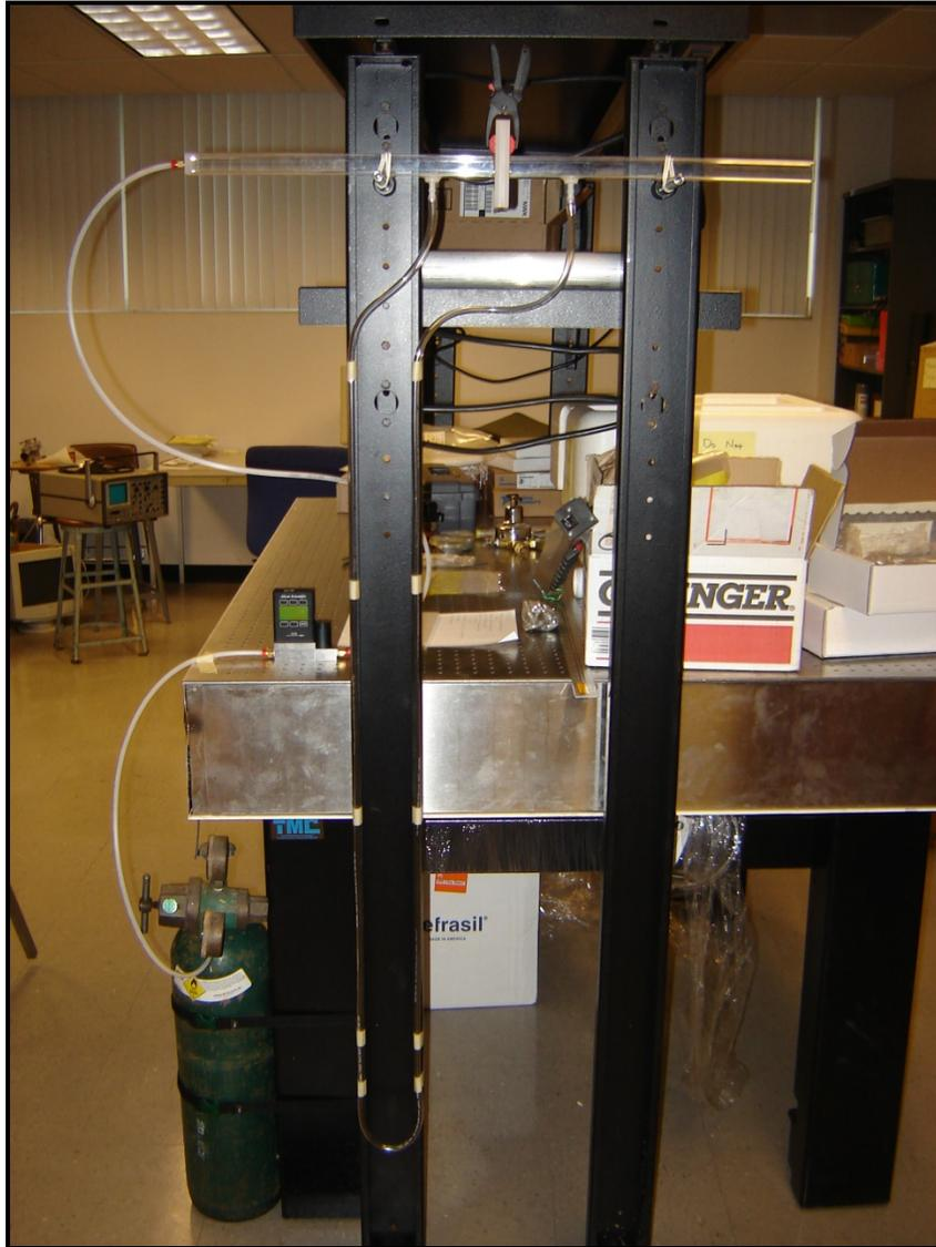
Fig. 20. Test setup including mass flow controller and liquid manometer (Gas was replaced with nitrogen cylinder)
