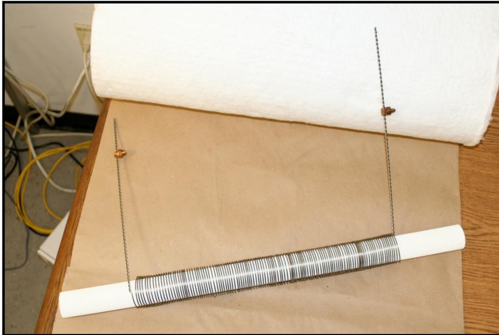
Fig. 12. Kanthal heating coil installed around outside of ceramic tube.
