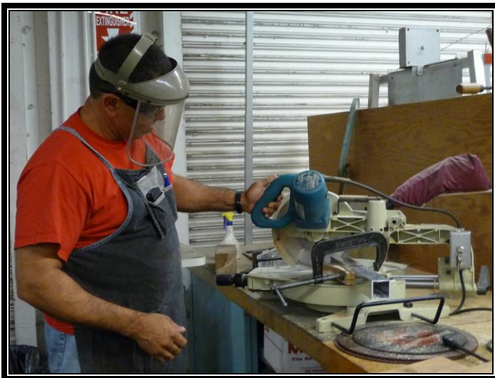
Figure 11: Chop saw and angle jig.
