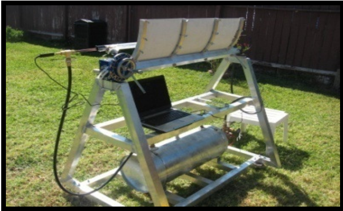
Figure 1: The solar collector trough has thermocouples attached to the computer.
