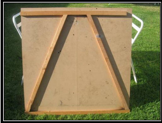
Figure 12: Welding jig fabricated from particle board.
