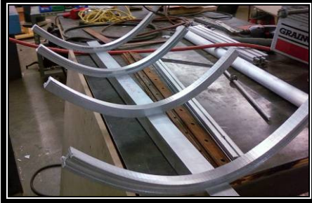
Figure 28: Curved coupon holder inset into pivot.
