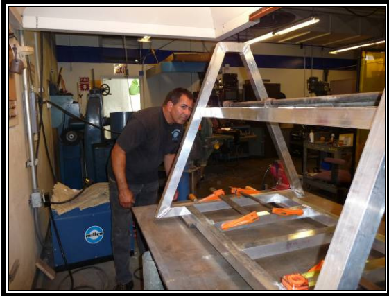
Figure 14 Alignment and clamping before welding.
