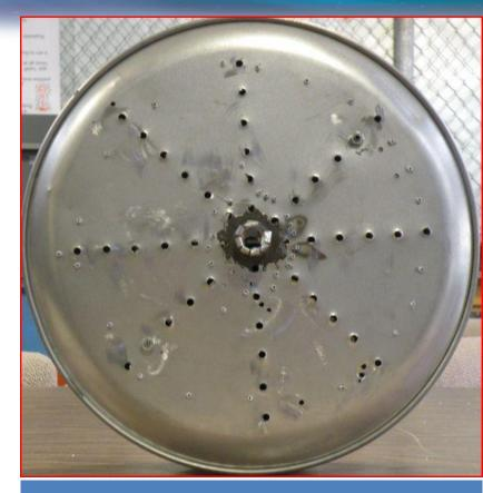
Heat recovery Wheel with drilled holes for smooth flow rate.
